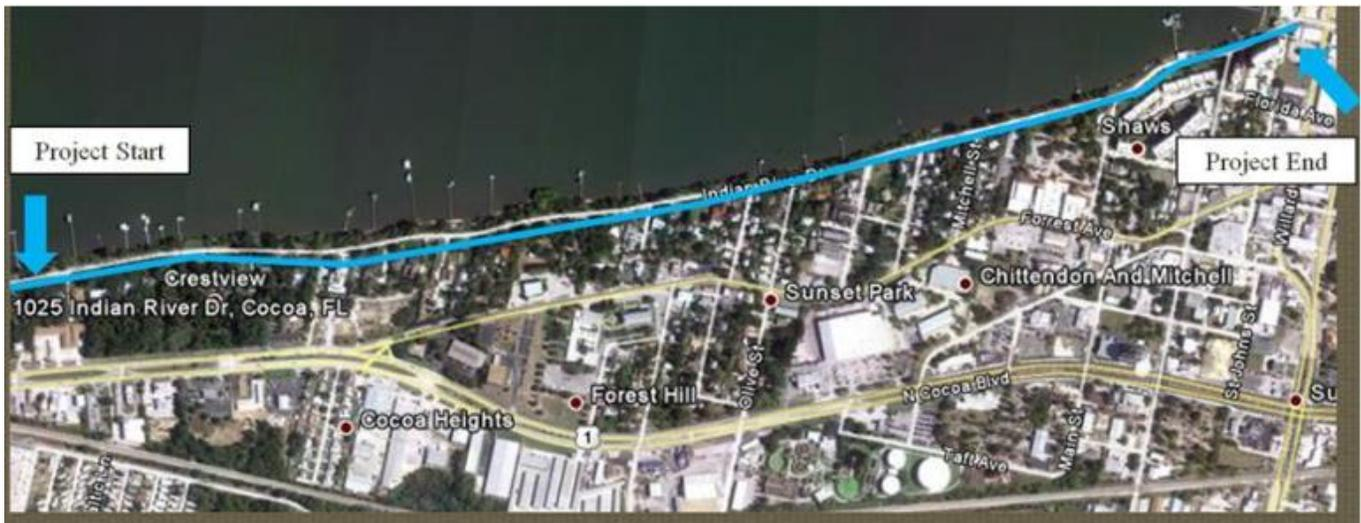
approximately 7,500 feet of existing six inch cast iron pipe and asphaltic concrete pipe, along with all the associated fittings and valves, with new 8" ductile iron pipe (DIP). All the fire hydrants and service lines will also be replaced.
